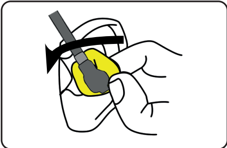
Carefully remove earpiece with index finger & thumb by gently twisting forwards.
